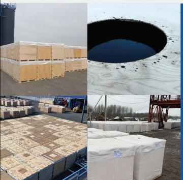
The dimensions of the container when assembled are 1060x1060x1095 mm. The capacity is up to 1040 kg of hot bitumen of various thicknesses. The heat resistance of the package is up to 200 degrees. The container is made only of glued material — FC plywood, glued in a checkerboard pattern. This eliminates the need to process and install the ISMP15 stamp during export.
